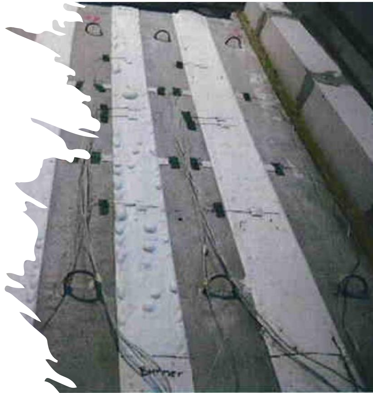
Linear joint seal installed for fire testing
